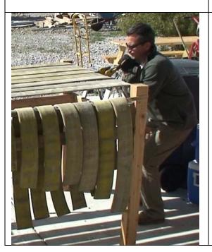
Once the fire hose is attached on both ends, roll the metal pole to stretch the hose.
