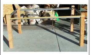
Put the metal poles into the drilled holes to make a hammock frame, and hold it together using a cargo strap
