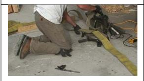
When cutting the fire hose, add 16 extra inches to the actual width and length of the hammock frame. This is needed so you can roll the fire hose on the metal poles.
