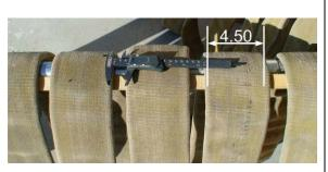
For example: pole length= 66 in. fire hose width= 4.5 in. divide 66 by 5.5 = 12 pieces of fire hose
