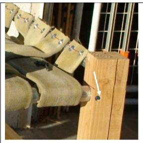
Then secure the metal pole to the 4x4 wood with a screw or bolt, so the metal pole can no longer move inside the hole.
